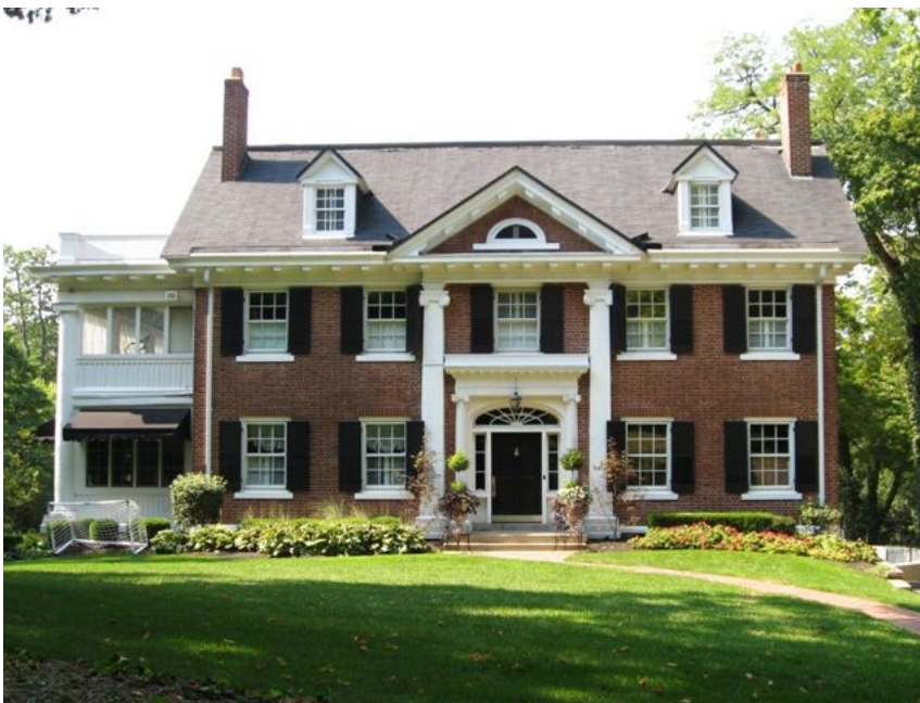
Georgian Revival Home with fanlight and sidelights on the main entryway door.
